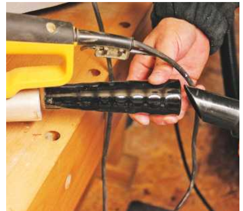
▲ A simple tapered adapter is supplied for power tools
